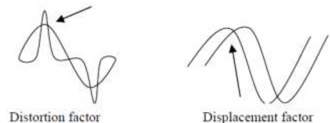
Figure 4.2 Distortion & Displacement factor
